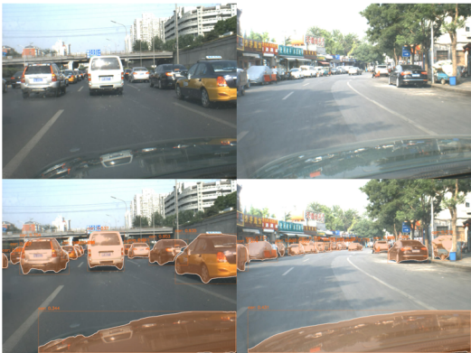
Fig. 3. The segmentation results of Bi-YOLOv8-seg on the TRoM dataset
