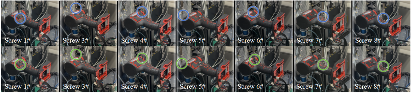
Fig. 7: Disassembly of Screws 1# and 3#–8#. Blue: Initial screwdriver position; Green: Successful disassembly.
