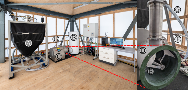
Fig. 1: Experimental setup for hydration of CaO with storage silo (A), buffer storage (B), motor (C) and the reactor (left). View into the reactor (right) [11].
