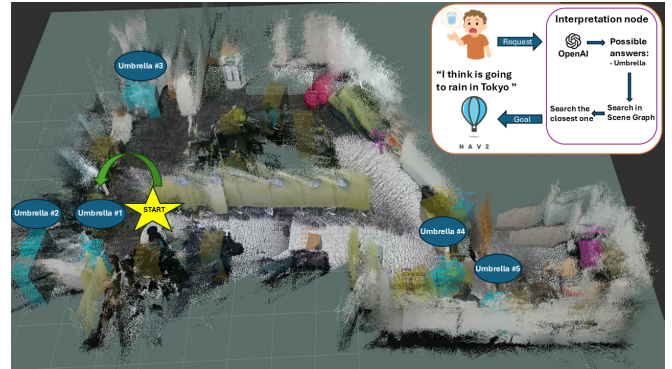
Fig. 3: Logic of the interpretation node: it interprets user requests, searches the scene graph, and sends a goal to the nearest matching object. Cyan markers in the 3D map indicate detected umbrellas.
