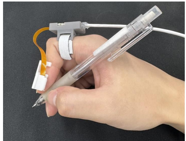
Fig. 1 Demonstration of the proposed wearable tactile sensor in a writing task
