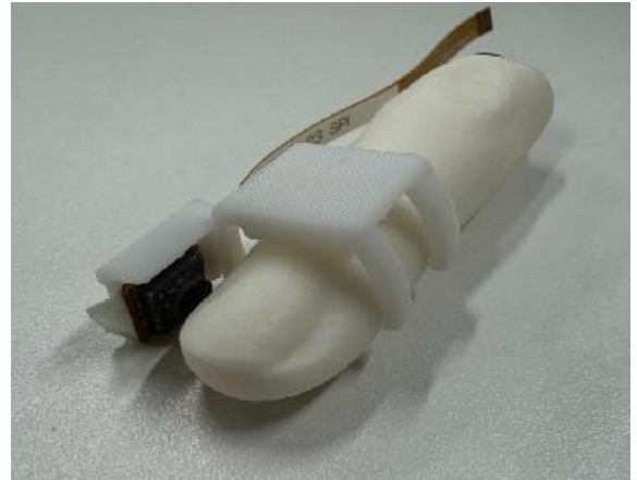
Fig. 3 Tactile sensor and fixture designed for measurements.
