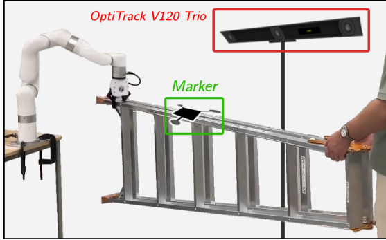
Fig. 5: Configuration of the Motion Capture System
