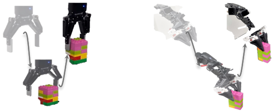
(a) Grasp-and-lift task performed by an UR5 robot with an Robotiq 2F-140 gripper. (b) Grasp-and-lift task performed by an ALOHA robot with the standard ALOHA gripper.
