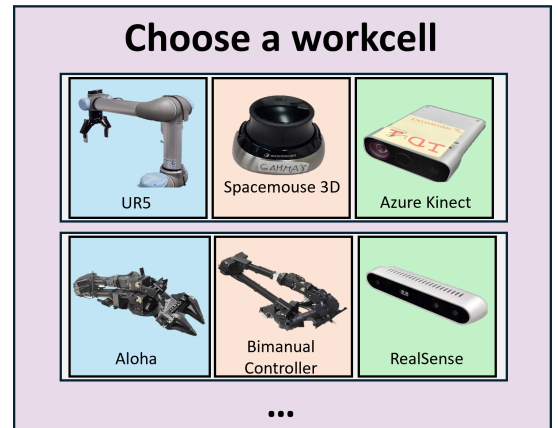
(b) Examples of specific workcells: one with a UR5 manipulator, a SpaceMouse controller, and Azure Kinect cameras; another with the ALOHA bimanual platform, its dual-hand controller, and Intel RealSense cameras. The ellipsis indicates that additional workcell configurations can be supported.
