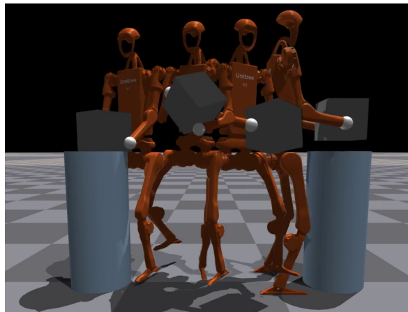
Fig. 1: Loco-manipulation with H1 to transport a box from the right pillar to the left one using a single policy trained in simulation with constraints as terminations.
