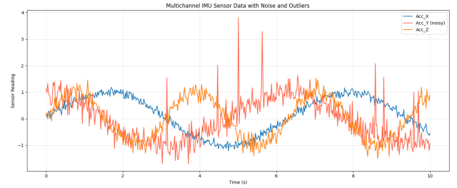
Fig. 1: Depicts the three accelerometer axes - Acc X, Acc Y, and Acc Z, highlighting that Acc Y shows increased noise and outlier spikes, indicating sensor disturbances or data corruption.
