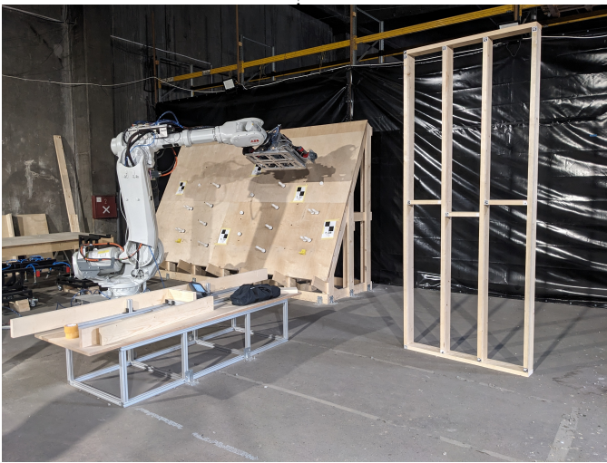
Fig. 3: Robotic panel assembly system with an example of panel.
