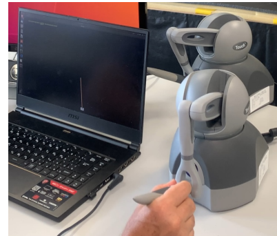
Fig. 2: The experimental interface is shown. The setup allows delivering passive replay of prerecorded control trajectories through the haptic device held by the users. Alternatively the users can control the cart-pole in real-time.
