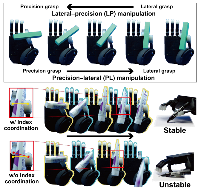
Fig. 1. PL and LP in-hand manipulation. To effectively support the thumb’s force, the index finger shifts its position using motor current feedback, as illustrated by the change from the red (without (w/o) the use of the index) to the yellow (with (w/) the use of the index) line in the red insets. This enables both stable object manipulation and a firm grip for tool use (w/ index), whereas a lack of coordination leads to grip failure (w/o index).
