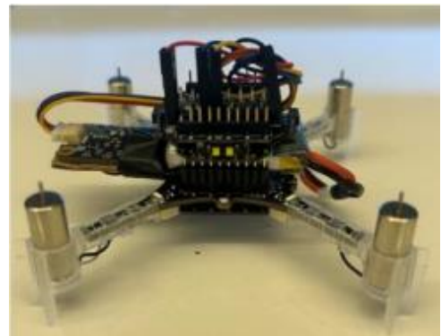
Figure 2. Fully assembled drone with expansion deck sensors and thermal sensors attached.
