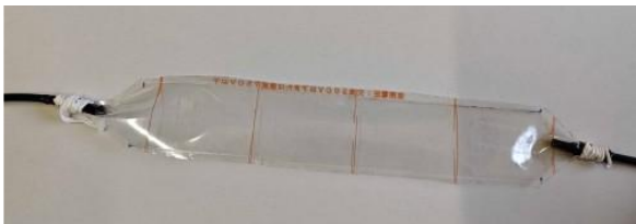
Figure 8. Polyurethane channel used as the control condition in human trials
