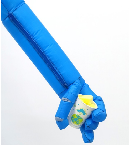
Fig. 13. Grasping a paper cup, holding a total weight of 14 g.
