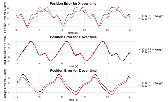
Fig. 5: Position tracking error comparing the case with and without unmodeled load, both running with ID + PF.
