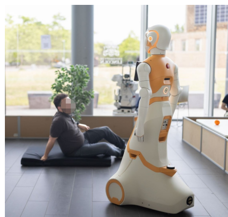
Fig. 1. ARI social robot approaching a participant simulating a fall during system evaluation.
