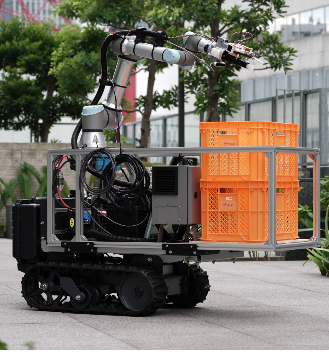
Fig. 2: Proposed Citrus unshiu Harvest Robot System
