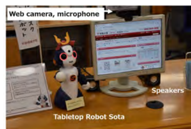
Fig. 3. Overview of experimental robot system at library helpdesk counter.
