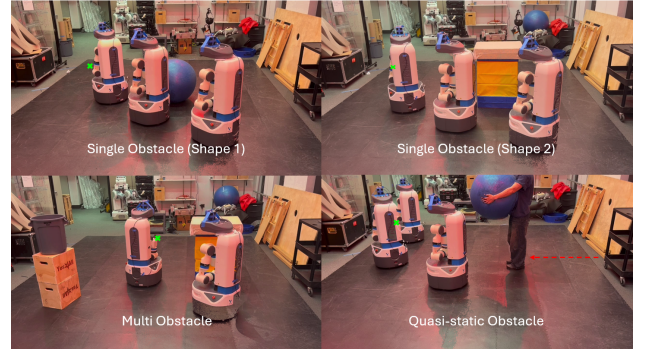
Fig. 8: Real-world experiments. Shown are collision-free RNBF-CBF-QP trajectories overlaid on video frames for static (single obstacle - shape 1 & 2, and multi obstacle) and quasi-static obstacle scenarios.
