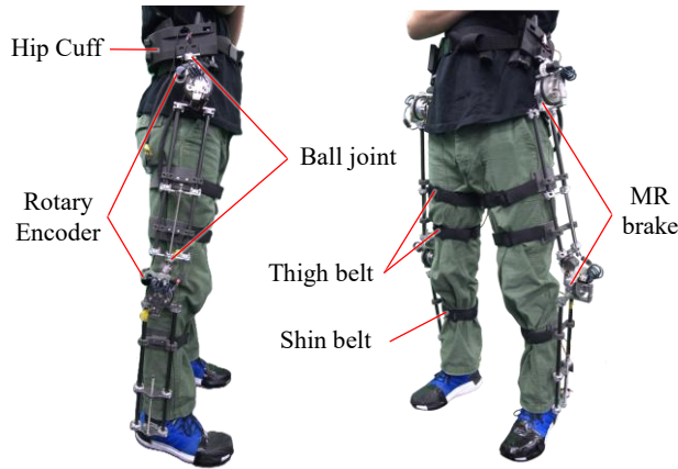
Figure 1. Overview of a lower limb force feedback exoskeleton.
