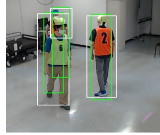
Fig. 7: Example of input Bounding Boxes and predicted Bounding Boxes(white square:input bounding box, green square:predicted bounding box).
