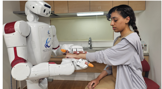
Fig. 1. The humanoid robot AIREC measures the radial pulse at the human wrist via a tactile sensor embedded in its palm. During measurement, one hand supports the human wrist, while the other gently applies pressure to stabilize it.
