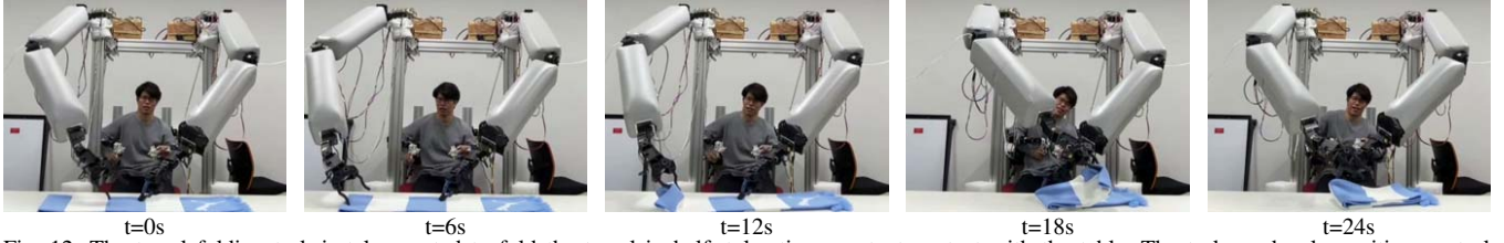
Fig. 12: The towel folding task is teleoperated to fold the towel in half, tolerating constant contact with the table. The task used only position control based on the feedback from the human operator’s vision, with no force feedback. Incidental contact happened with the table and between the arms, which did not result in any servo faults.
