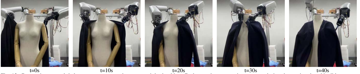
Fig. 13: Coat assistance task helps to put a coat on the mannequin’s shoulders. Both arms have come into contact during the motion, but this did not stop the teleoperation, as the impact was absorbed by the robot’s compliant body.
