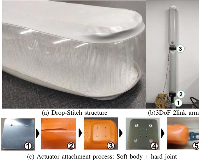
Fig. 2: (a) To visualize the Drop-Stitch structure of the Transparent balloon sample. (b) The design result of base (1), shoulder (2), and elbow (3) servo joints from the result of 3DoF 2link inflatable robot payload test [29] (c) Interconnection process for soft body to rigid joint. (1) With an adhesive, the balloon plate (1) is fixed to a fabric piece (2), then attached to the balloon (3). Another metal plate called "mediator plate" (4) connects the soft body (inflatable link) with the rigid joint (servo frame) (5) [29].
