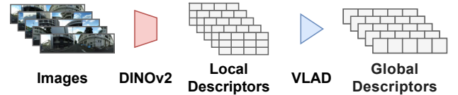
Fig. 2. Feature extraction using AnyLoc-VLAD-DINOv2.
