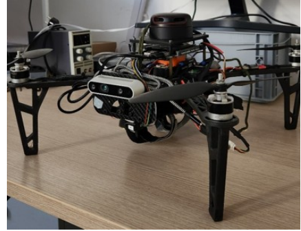
Fig. 6: Drone used during experiments equipped with IMU sensor integrated into the camera, 2D LiDAR positioned above the drone, and range finder positioned underneath the frame.
