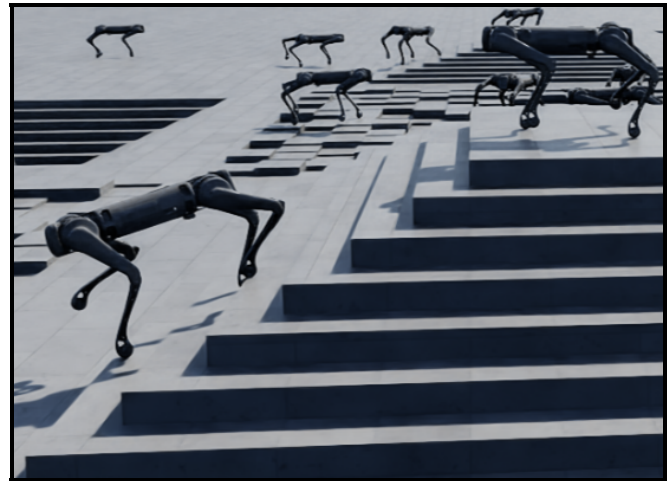
Fig. 1. Unitree B1 walking down stairs in Isaac Sim using a torque-driven RL locomotion controller.
