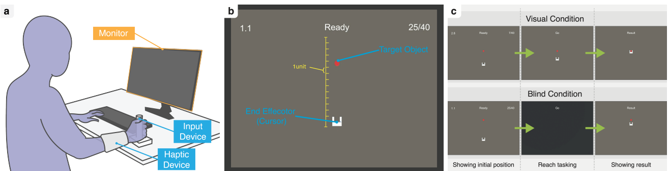
Fig. 3. (a) in the setup, participants use an input device and wear a haptic device, (b) the monitor shows a target and a cursor, (c) the task sequence and displayed information differ by visual condition.
